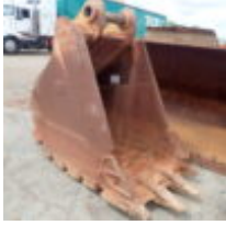
1050MM TRENCH BUCKET TO SUIT 330/336 EXCAVATOR | Stock No. 6/7196
