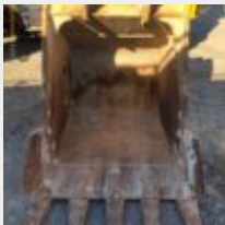
1000MM EXCAVATION BUCKET TO SUIT 320D | Stock No. 6/7014
